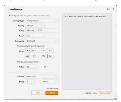
Figure 9k - Message addressed to a circular area
