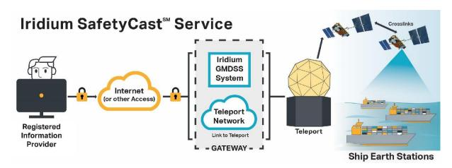
Figure 2 – Basic concept of the Iridium SafetyCast service
